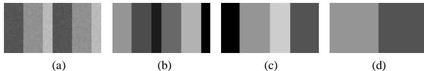
Fig. 2. (a) is a greyscale image. (b), (c), and (d) shows segmentations of the image with \delta = 97\% , 98\% , and 99\% , respectively
